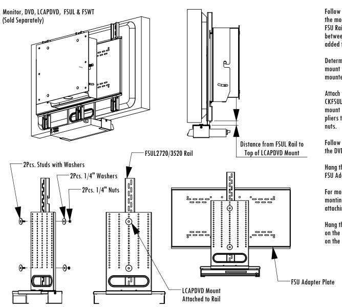
Follow the FSU Installation Instructions for attaching the monitor to the FSU Adapter Plate. When attaching FSU Rails to the monitor add an additional washer between the monitor and FSU Rail to allow for the added thickness of the LCAPDVD mount.
